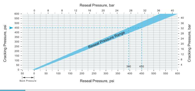
All valves are factory tested for cracking pressure and reseal performance.
