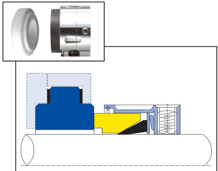
Component seal with multiple springs
