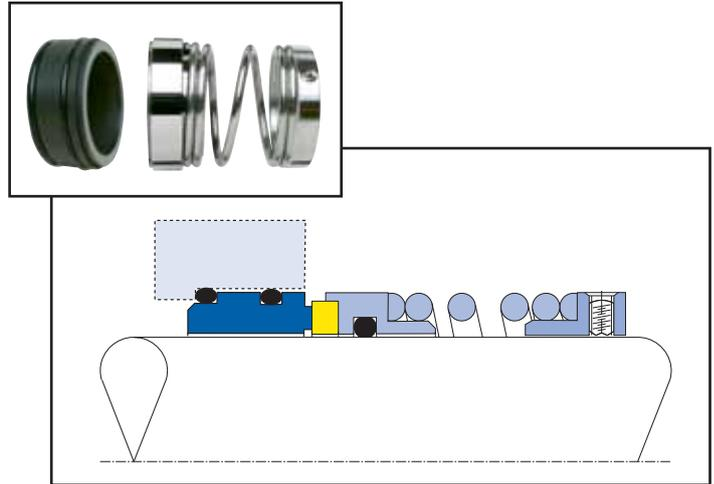
Component seal with single coil spring
