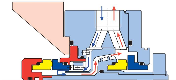
UHDDS™ Tapered Vane Circulating Device.
