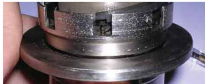
Above: Example of one type of rotary seal face drive. Rejected for use in AESSEAL® designs
