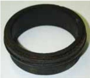
Typical seal component fitted to test separator pump in the North Sea, showing signs of sand wear.
