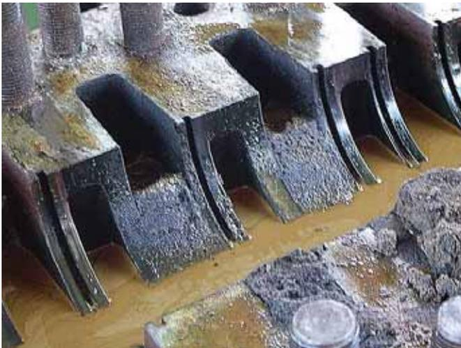
Sulzer MSD 4x8x10.5 bottom half casing showing severe sand accumulation
