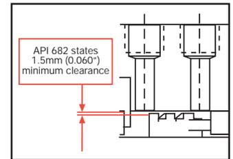
Parallel Helical Vane (Screw) Circulating Device.
