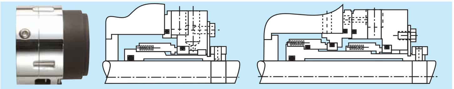
Non-AES API 682 Single & Dual seal configuration with multiple springs positioned in the process media.
