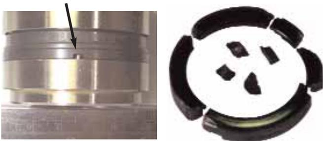
Above: Example of one type of rotary seal face drive. Rejected for use in AESSEAL® monolithic seal designs.
