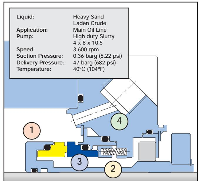
2.635" CAPI™ A1 Single Seal fitted to Multi-stage pump in Nigeria
