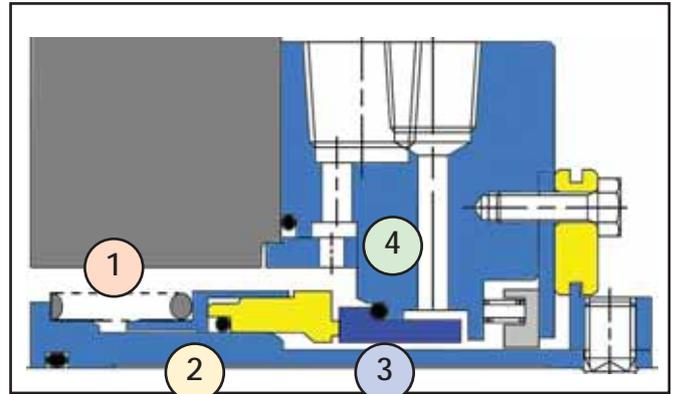
Typical seal installed with the problem areas highlighted
