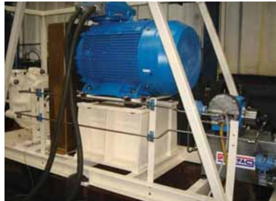
CAPI A1 Dual seal on a Warman Slurry pump
