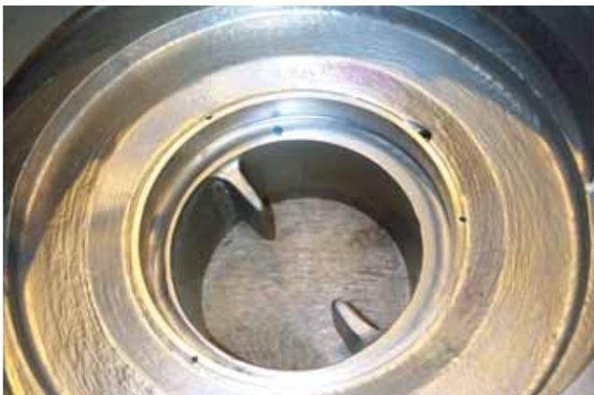
A worn volute casing caused by sand erosion on an API 610 OH2 MOL booster pump
