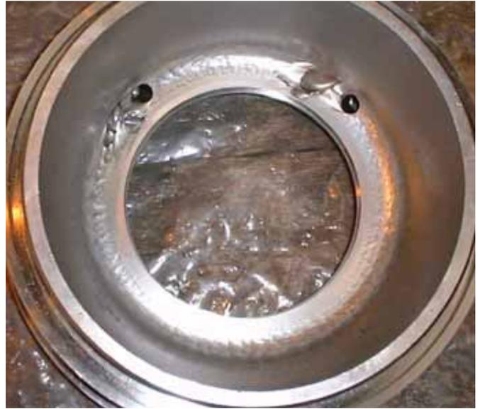
Non-AES seal gland plate showing signs of sand erosion due to process fluid vortexing
