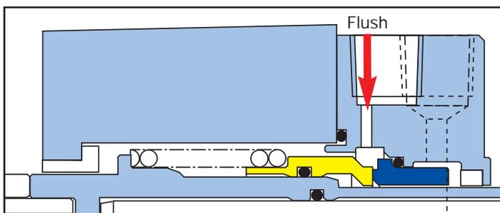
Non-AES Single Seal Design with flush port directly over the seal faces
