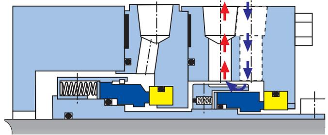
Non-AES seal design with a "Parallel Slot" Circulating Device.
