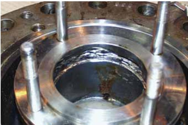
Damage to the stuffing box of a multistage centrifugal MOL Pump
