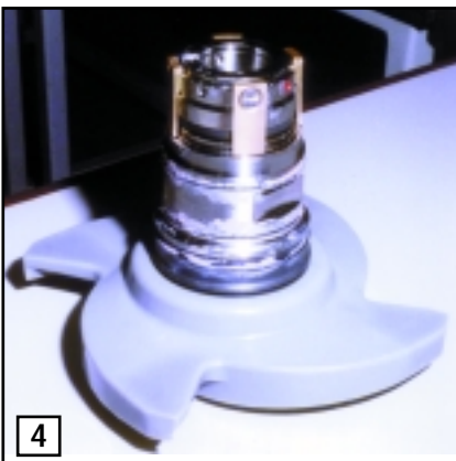
4 Fit the seal inside the impeller, ensuring the impeller anti rotation pin locates in the recess in the seal.
