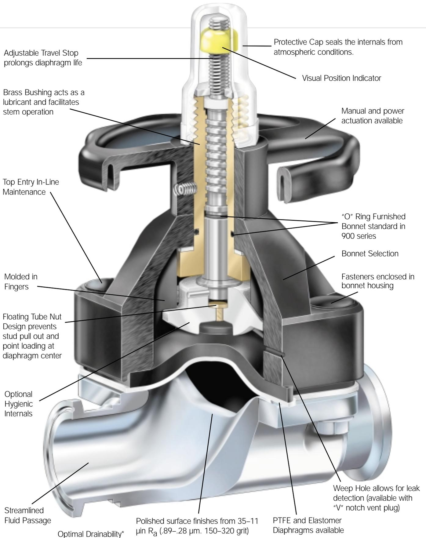
\*Schedule 5, 10 and 40 butt weld valves are not drainable in a horizontal line.
